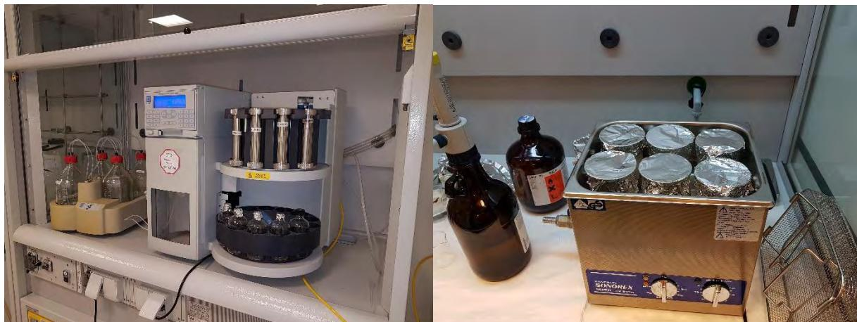
Figure 19: Cells extraction on ASE system and filter extraction on USE system
