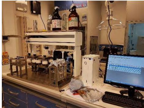
*Figure 13: Filter elution on automatic extractor*
