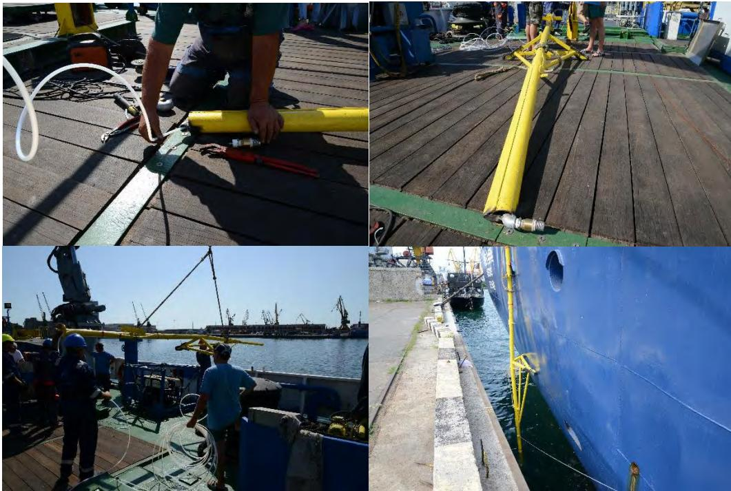
*Figure 14: Sampling metal probe mounted on hull of the ship*
